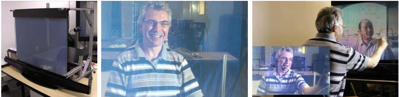
Figure 1: (a) Prototype system with part of enclosure removed, (b) captured image showing interference from backscattered projected image, (c) system in use with notch filter on camera (inset shows captured image, mirrored, sent to remote user)
